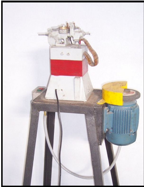
Butt Welding Machine with grinder for 2.5mm to 0.8mm
